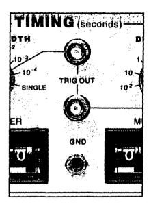
TRIG OUT (LOWER): This BNC connector provides a signal which is coincident with the Duration timing signal which controls pulse output.
