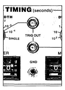
TRIG OUT (LOWER): This BNC connector provides a signal which is coincident with the Duration timing signal which controls pulse output.
