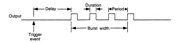
**DELAY:** These controls set the time between the initiating trigger event and the beginning of the pulse burst. If this rate selector is set to **NONE** or the multiplier is set to **0.00** there is no delay.
