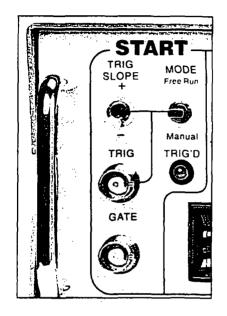
**GATE:** This BNC connector allows a signal from an external source to restrict the final output signal. This input must be at a logical high (or open-circuited) in order for the *Model 2100* to recognize either manual or automatic trigger events.
