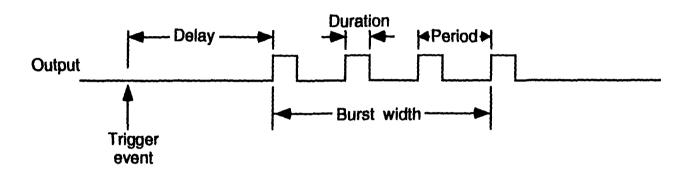
**DELAY:** These controls set the time between the initiating trigger event and the beginning of the pulse burst. If this rate selector is set to **NONE** or the multiplier is set to **0.00** there is no delay.
